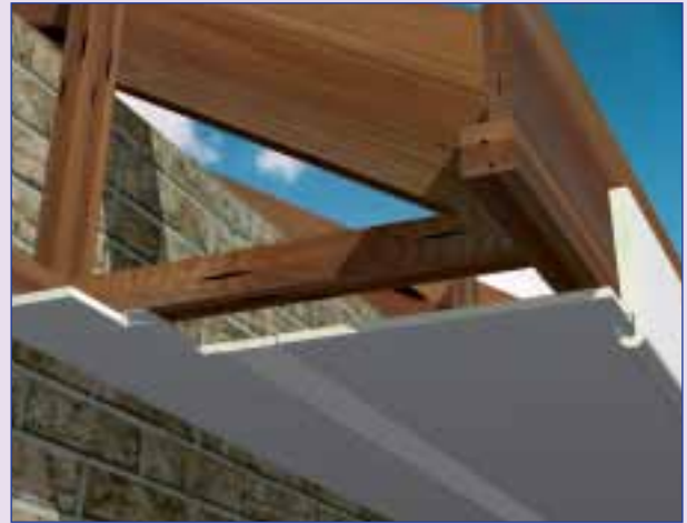
18mm Bullnose Fascia – Vented multi-purpose board as a soffit
